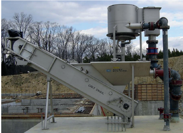
Figure 7.5 High performance Eutek SlurryCup™ grit washing/sludge degritting unit mounted on a Eutek Grit Snail quiescent dewatering Escalator. Source: Courtesy of Hydro International.
