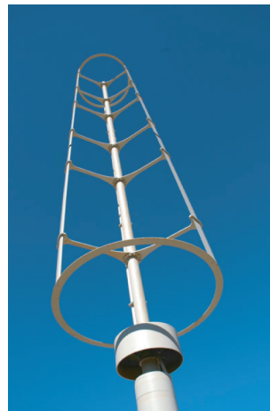
Figure 10.13 Vertical axis wind turbines. Source: http://science.howstuffworks.com/environmental/green-science/wind-power2.htm , http://news.cnet.com/8301-11128_3-9956965-54.html , http://windturbinezone.com/wind-turbine/vertical-wind-turbine . All reproduced with permission.
